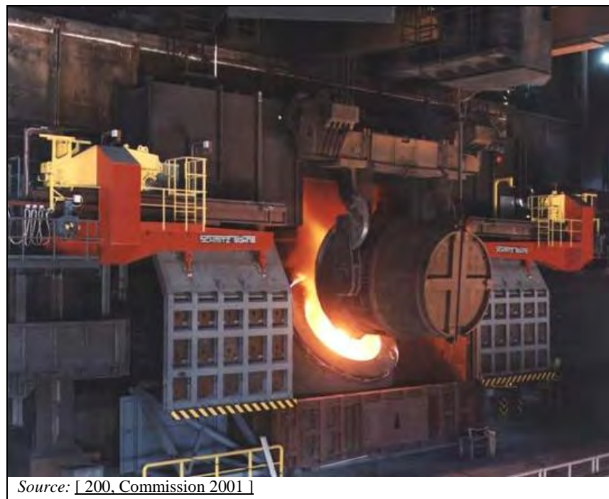
Figure 7.1: Basic oxygen furnace at the moment of charging hot metal
