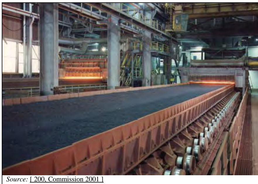
Figure 3.1: Photograph of a sinter strand with the charging facility (drums or chutes) and the ignition canopy at the starting end
