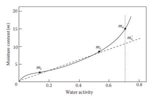
**FIGURE 12.4** Schematic of a typical moisture sorption isotherm for breakfast cereal with a superimposed straight line of slope *b*. Initial  $(m_i)$ , critical  $(m_c)$  and equilibrium  $(m_e)$  moisture contents are indicated together with the pseudo-equilibrium  $(m'_c)$  moisture content used for package shelf life calculations.
