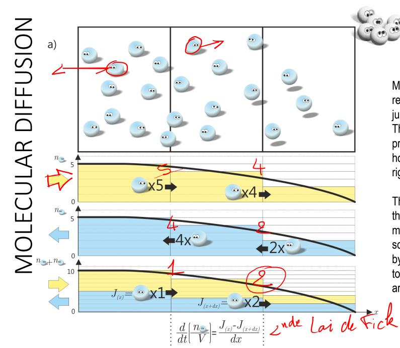
Molecules are represented as jumping beads. They have equal probabilities to hop to left and right directions.
